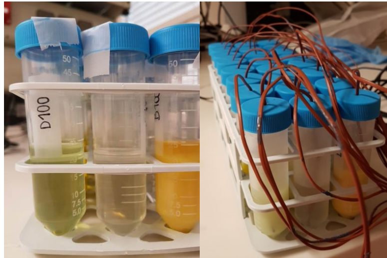
Fig. 1. Preparation of the tube rack with the fuel blends to be frozen; the caps have been bored in the middle to insert a thermocouple in each tube
